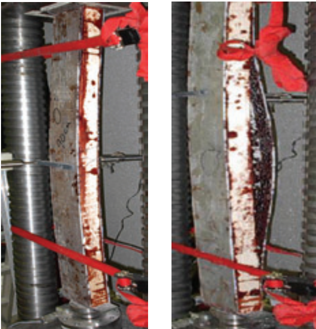
In-phase and out-of-phase delaminations of GFRP reinforced Glulam columns
